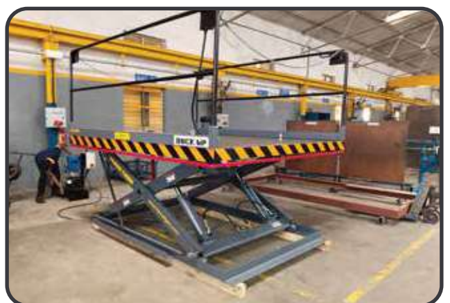
Platform: 2.5m X 2m | Stroke: 1.6m | Capacity: 2T
