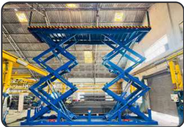
Platform: 4m X 2.5m | Stroke: 2.3m | Capacity: 6T
