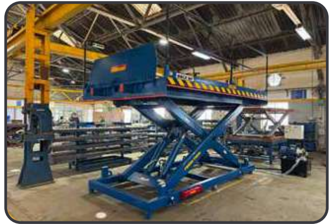
Platform: 4m X 2.5m | Stroke: 2.3m | Capacity: 6T
