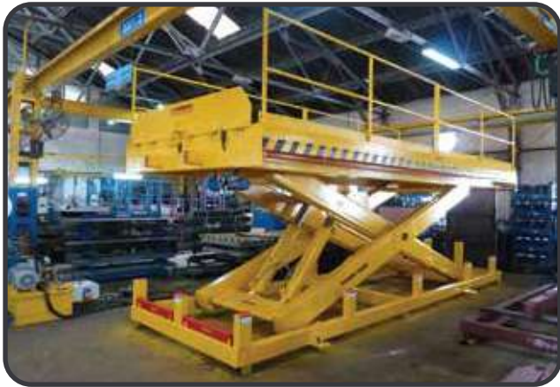
Platform: 6m X 2.5m | Stroke: 2.6m | Capacity: 12T
