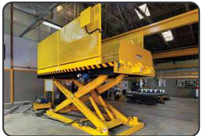
Platform: 5m X 2.5m | Stroke: 3m | Capacity: 3.5T
