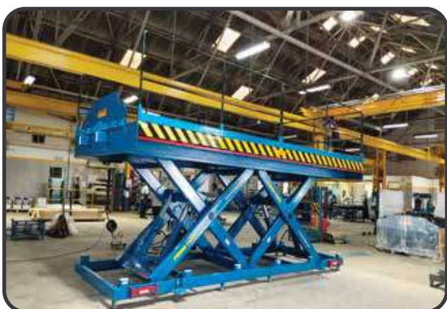
Platform: 6.5m X 3m | Stroke: 2.5m | Capacity: 6T
