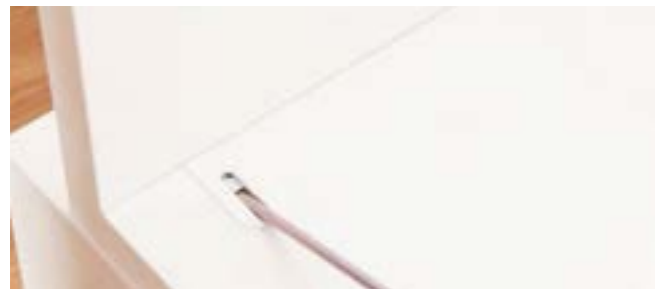
Join furniture elements with cordless drill and Cabineo tool. Easy, fast working with preset torque approx. 2.5 Nm.
