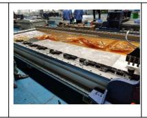
The worktable has the selfgrooving function which can groove the worktable surface to get better accuracy
