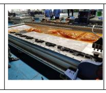
The worktable has the selfgrooving function which can groove the worktable surface to get better accuracy
