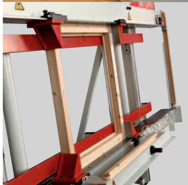
LETTURA PEZZO IN AUTOMATICO TRAMITE FOTOCELLULE AUTOMATIC WORKPIECE READING THROUGH PHOTOCELLS
