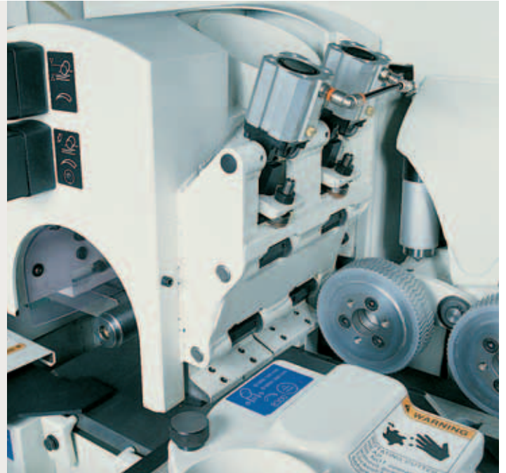
Receding chip breakers on top horizontal spindles with pneumatic pressure
