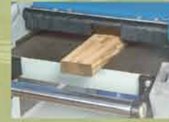
Anti kickback system to avoid back sliding
