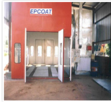
Complete Paint Booth with Civil Basement with Insulated Panel
